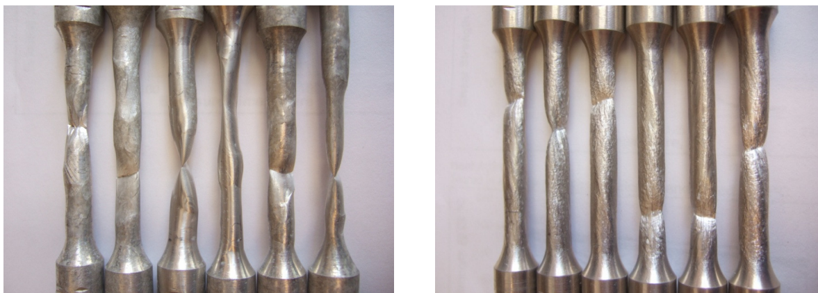
Figure 84: Al5N (left) and Al5NFeSi (right) specimens after tensile tests.
