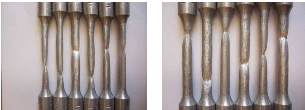
Figure 85: Al2NFeSi (left) and Al2NFe2Si (right) specimens after tensile tests.
