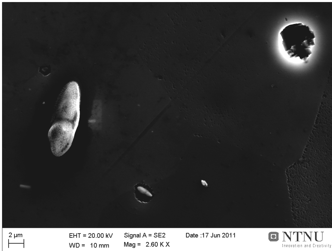
Figure 79: Small particle found in alloy Al 2 NFeSi, located in the lower part of the image slightly left of the centre.
