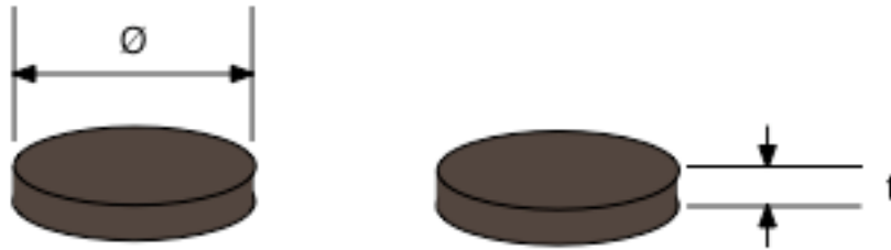
Figure 52: Pellet geometry represented as a perfect cylinder with diameter \emptyset and height t .
