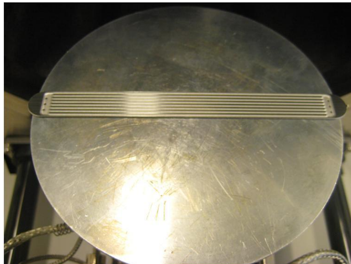
Figure 22: The bipolar plate attached to the sample table by carbon stickers.
