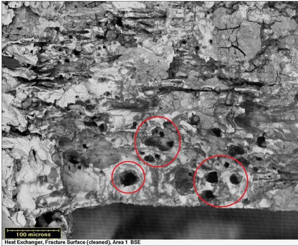
Figure 7: SEM (Backscatter mode) image showing pitting corrosion in 300 stainless steel [13].
