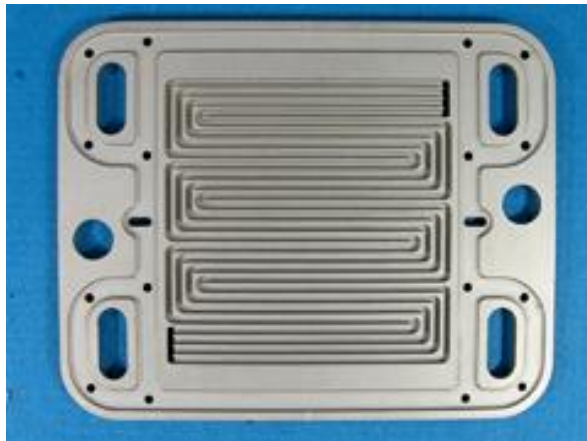
Figure 3: Nitrided metallic bipolar plate. The plate conducts the current between each cell in a stack, and the flowfield leads the gas through the cell. [9]
