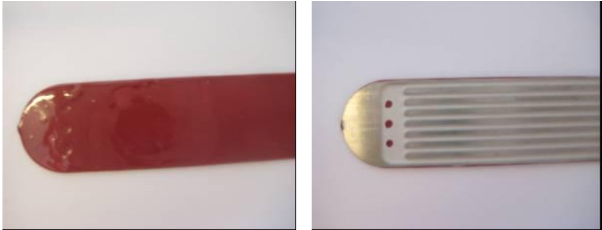
Figure 17: a) Stainless steel plate coated with nail varnish to avoid corrosion on both sides. b) The front side of the bipolar plate which was not coated with nail varnish.
