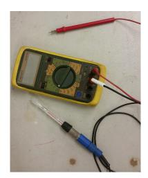
Figure 19: Setup of corrosion potential measurement.
