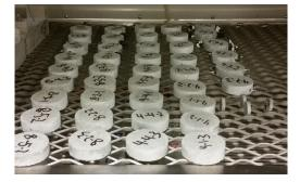
Figure 14: Bottles sawn into discs, placed in carbonation cabinet.
