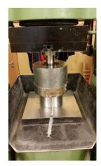
(a) The machine used for pore solution extraction.
