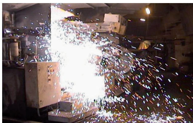
Figure 6.2: Sparks released into the tapping area from the furnace taphole due to gassing phenomenon in a silicon production furnace.
