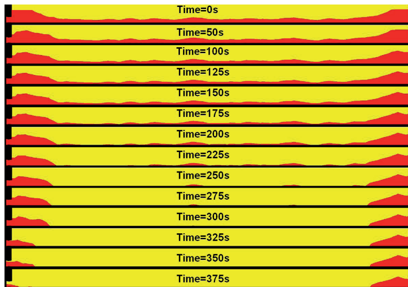
Figure 5.18: Evolution of the metal pattern in the lower part of the central plane of the ferrosilicon furnace which explains the reason for the sudden flow rate drop during furnace tapping.
