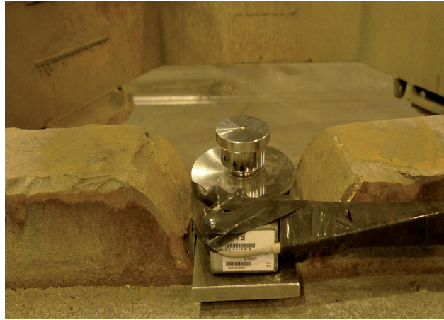
Figure 5.28: One of the load cells installed on the weighing panel before the tests at Elkem Salten plant, April 2010.
