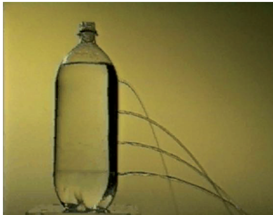
Figure 3.4: The effect of liquid height on the exiting flow rate from the holes made on the surface of a bottle of water.
