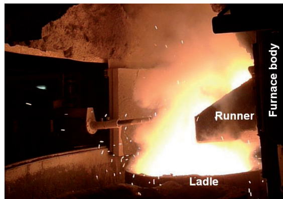
Figure 3.2: A side view of tapping of silicon melt from a submerged arc furnace, very high temperature melt flows into the ladle from the furnace hearth.
