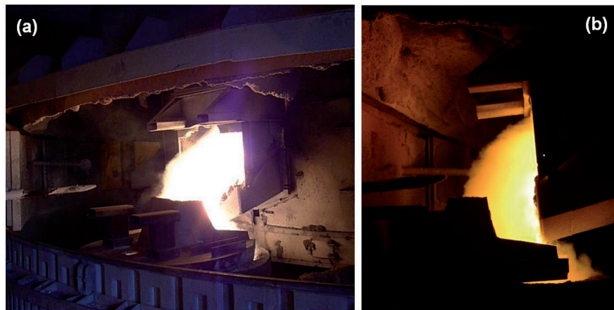
Figure 6.36: Successful performance of the hood system using the lid over the ladle during tapping in a silicon furnace at Elkem Thamshavn plant.
