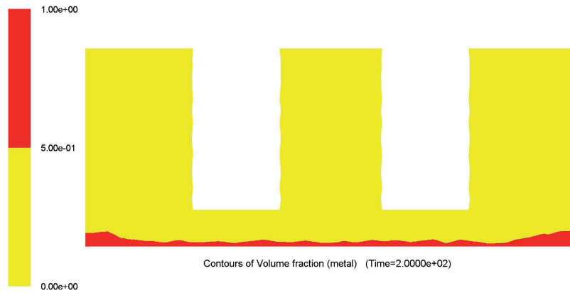
Figure 5.13: 2D contours of metal volume fraction in a vertical plane including two electrodes inside the silicon producing furnace.
