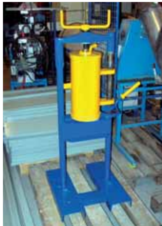
Fig. 4.10: Filter press used in making the \text{AlF}_3 filter grains
