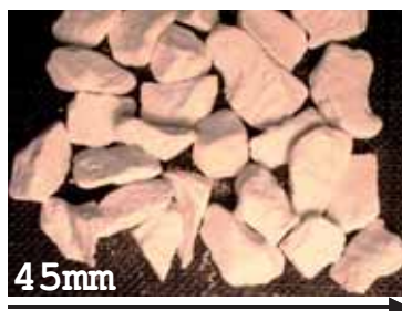
Fig. 4.15: Filter grains acquiring their irregular shape from crushing of sintered filter cakes.
