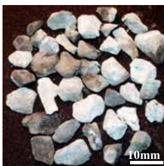
Fig. 5.7: Spent filter material from the “active” \text{AlF}_3 filter
