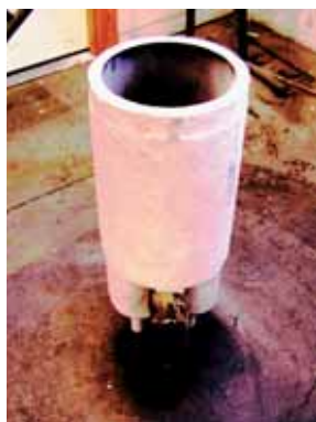
Fig. 5.4: Complete filter setup in the cast shop
