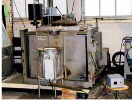
Fig. 5.6: Experimental setting consisting of furnace for melting and cylindrical furnace for preheating
