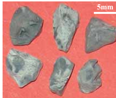
Fig 7.14 Morphology of jagged filter grains
