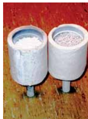
Fig. 5.5: left – passive filter unit ( Al_2O_3 ), right – active filter unit ( AlF_3 )
