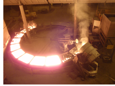
Figure 1: The silicon casting area. A ladle full of molten silicon is poured into trays, one by one as the trays rotate on the carousel.
