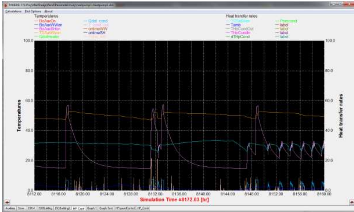
Figure 4.2. The online window from TRNSYS Type 65 makes it possible to show any value (Temperature, flow rate, heat rate, etc.) in the simulated system (screenshot from program).
