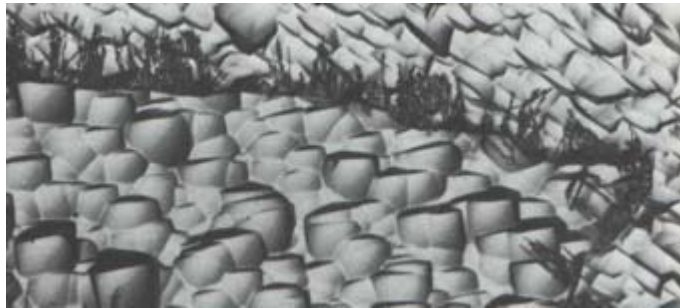
Figure 2•14: a) Optical micrograph of mold-cast Si , mechanically polished surface (35x), dots are SiC-particles b) Etched surface with SiC segregation (200x), from Dietze et al. [1981]
