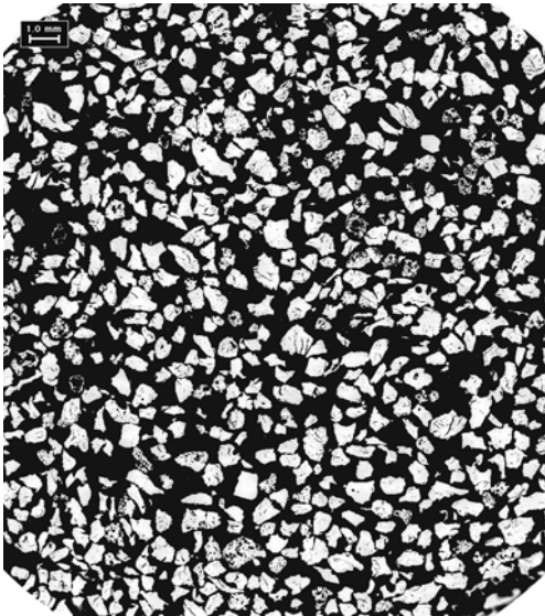
Fig. 4.1-2. Coke fraction 0.5-1.0 mm. Magnification 80 x, polarised light.
