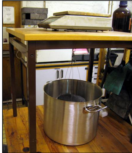
Fig. 3.6-1. Hydrostatic balance used for density measurements.
