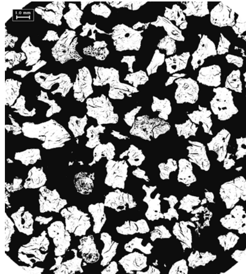
Fig. 4.1-4. Coke fraction 1.4-2.0 mm. Magnification 80 x, polarised light.
