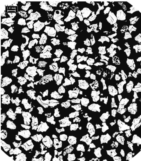
Fig. 4.1-3. Coke fraction 1.0-1.4 mm. Magnification 80 x, polarised light.
