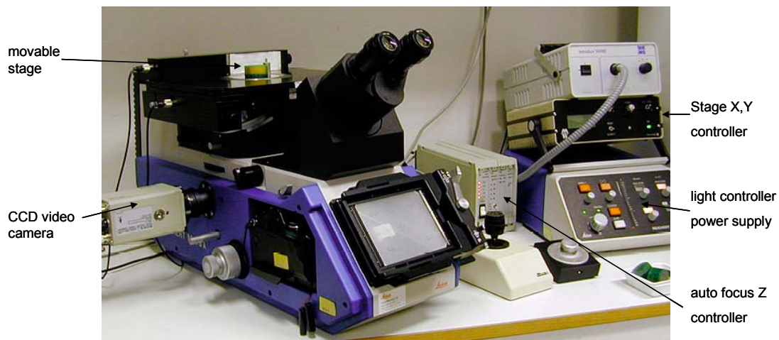
Fig. 3.5-2. Hardware setup used for optical microscopy and image analysis.
