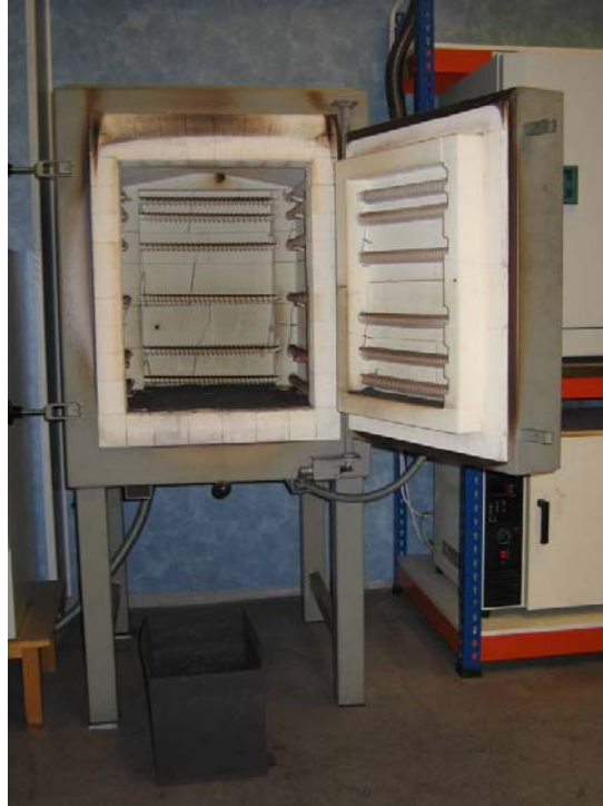
Fig. 3.4-2. Electrically heated oven (Nabertherm N 150/H) and steel container used for the baking of green anodes.
