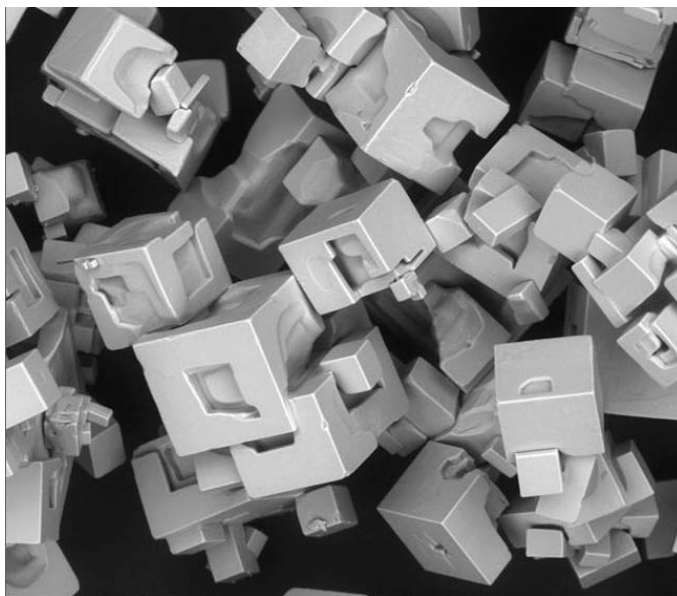
Fig. 1.2: NaCl crystals precipitated from water+MEG (~90wt % MEG), ~140°C. Size 20-100µm.
