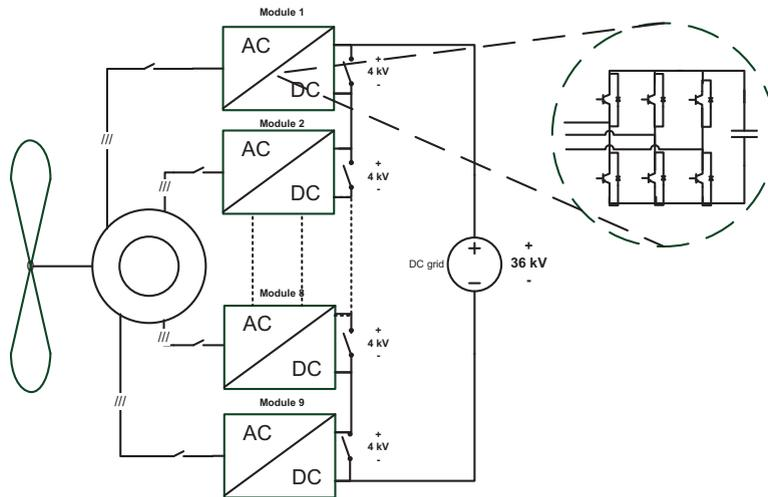
Fig. 1. Principal overview of the modular series connected converter generator drive
