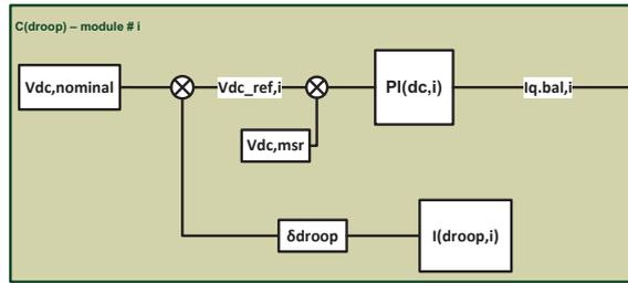
Fig. 3. Droop control scheme for DC-bus balancing
