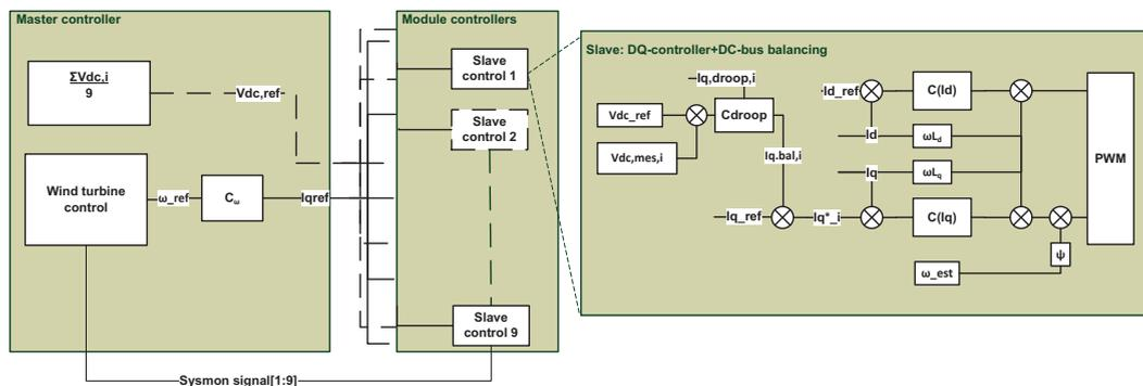
Fig. 2. Control system structure with master controller, slave controller organization and content in each slave
