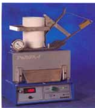
(a) (b) Figure 2. (a) PoDFA equipment [11]: the molten metal is poured in a crucible and placed on top of the vacuum chamber; (b) schematic illustration of the process: the metal is sucked by the vacuum and forced to flow through the porous filter disc which is cut and prepared for the microscopy investigation.
