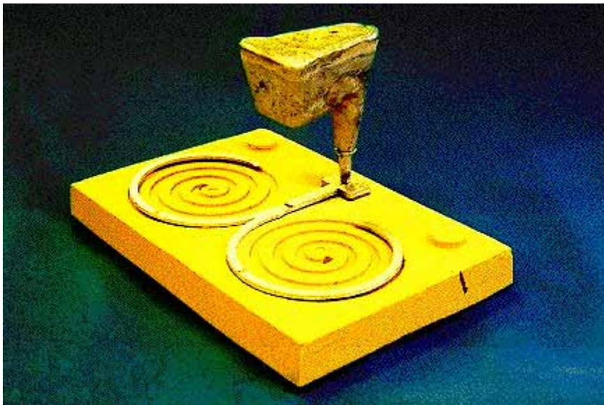
Fig. 2 Pouring basin and double-spiral mould of the original version of spiral fluidity test equipment.
