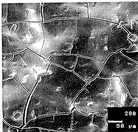
Figure 5.59: Ti/IrO_2 - Ta_2O_5 used in electrolyte with c(Mn^{2+}) = 10 \text{ g/l} for 50 hours. 200X.
