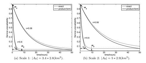
Figure 8: Log-plot of service unavailability E[U(t)] versus time t.
