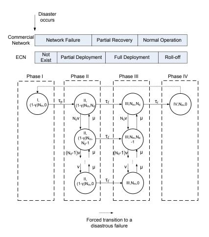
Figure 4: State transition diagram for the network operational stages.
