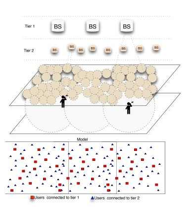
Figure 1: Illustration of a two-tier infrastructure wireless network utilizing two classes of BSs.
