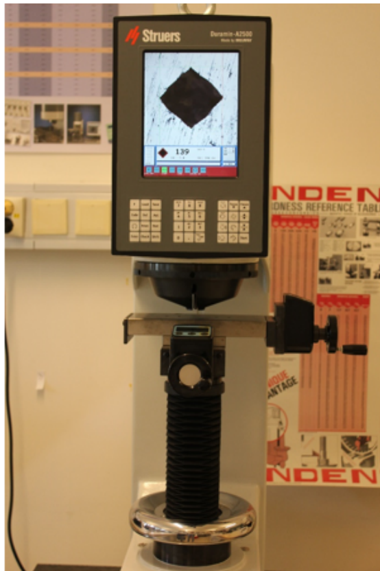
Figure 3.2: Picture of the Struers Duramin - A2500 used for measuring Vickers hardness.
