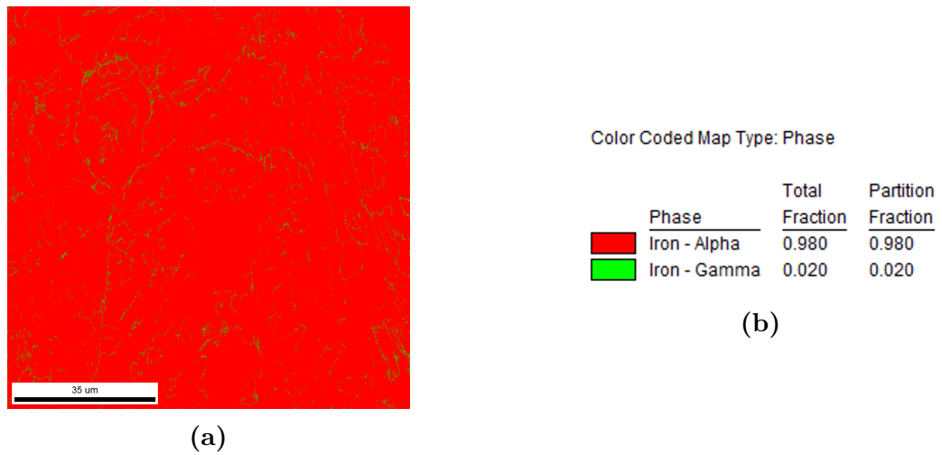
Figure 4.9: a) Phase map of base material where green areas represent FCC ( \gamma ) austenite and red areas represent BCC ( \alpha ). b) Fraction of BCC alpha and FCC gamma phase calculated by the TSL OIM Analysis software.
