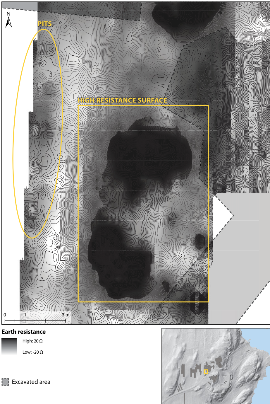
Fig. 16.17: Earth resistance plot over the south-western part of Area 5. Data collected by Earthsound Associates/NTNU 2009 (Barton 2010). Illustration: A. A. Stamnes, I. T. Bøckman, MCH.
