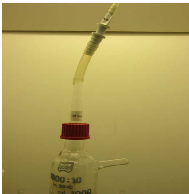
Figure 3.6 silicon pipe to connect CO 2
