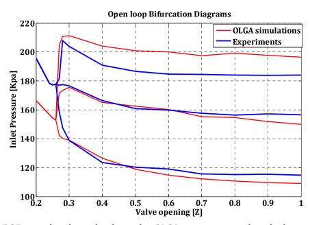
Figure 5.37: simulated results from the OLGA case compared with the experimental results from valve1. The bifurcation point is fairly the same for both models.
