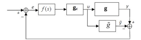
Figure 2.11: The internal model control (IMC) structure
