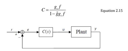
Figure 2.12: Closed-loop system with IMC controller (Jahanshahi and Skogestad 2013)
