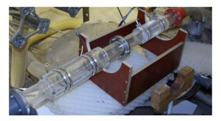
Figure 3.14: The conductance probe
