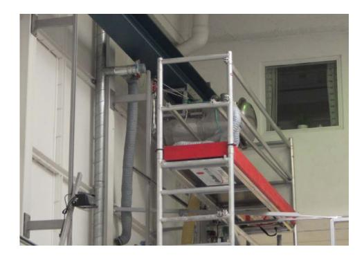
Figure 3.8: Over flow tank at top of riser
