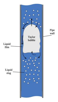
Figure 2.4: Schematic map of slug flow in a vertical pipe in a slug unit (Yan and Che 2011)
