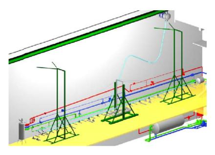
Figure 3.2: Multiphase Test Rig Layout, NTNU (Lilleby 2003)
