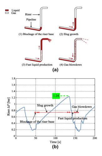
Figure 2.8: Stages for SS2 (a) a graphical illustration (b) marked on a cycle of an experimental riser  $\Delta P$  trace  $(U_{SL} = 0.10ms^{-1} \text{ and } U_{SGO} = 2.00ms^{-1})$  (Malekzadeh, Henkes et al. 2012)
