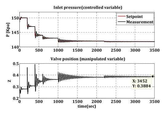
Figure 5.25: Simulation result of control by Shams's closed-loop method for the initial choke valve position of 30%. The values of Z=0.389 and P=142 kpa have been the maximum achieved valve opening and the minimum achieved set-point, respectively.
