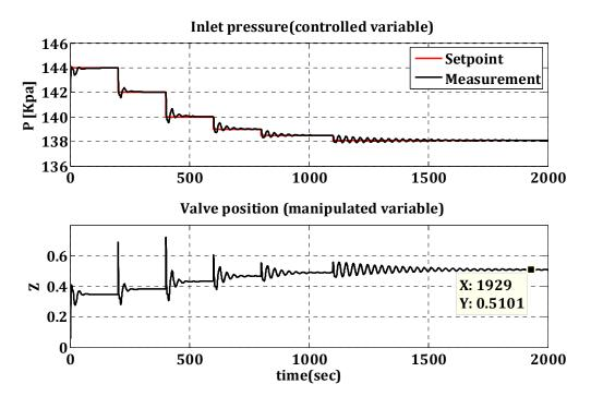
Figure 5.33: Simulation result of control using the IMC-based PI controller tuned at the initial choke valve position of Z=40%.
