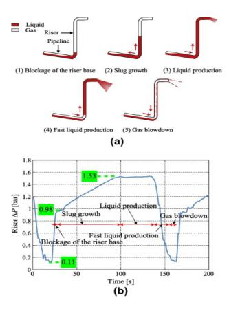
Figure 2.7: Stages for SS1 (a) a graphical illustration (b) marked on a cycle of an experimental riser  $\Delta P$  trace ( $U_{SL} = 0.20ms^{-1}$  and  $U_{SGO} = 1.00ms^{-1}$ ) (Malekzadeh, Henkes et al. 2012)
