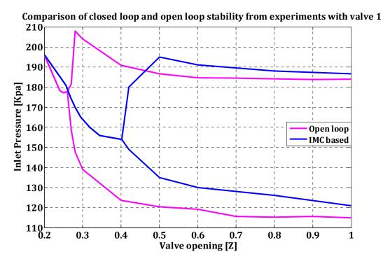
Figure 5.39: Comparison between the stabilizing control results from IMC-based tuning method and the open-loop system for the experiments with valve 1.
