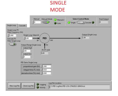
Figure 3.16: Implemented control modes in LabVIEW
