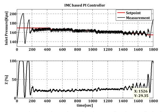
Figure 5.12: Result of control using the IMC-based PI controller. The controller has been able to move the bifurcation point from Z=16% up to Z=29.35%.
