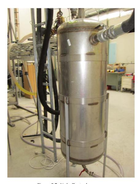
Figure 3.7: Air buffer tank
