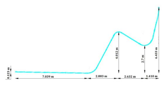
Figure 3.4: Configuration of the S-shaped riser test section (Lilleby 2003)
