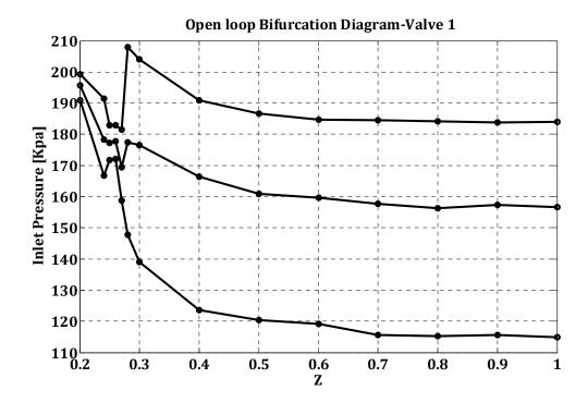
Figure 5.2: Open-loop bifurcation diagram from the slow choke valve experiments. The bifurcation point occurs at valve opening of Z=0.26. The top and bottom line illustrate the maximum and minimum values of oscillations for inlet pressure respectively at each operating point. The middle line shows the average values of pressure.
