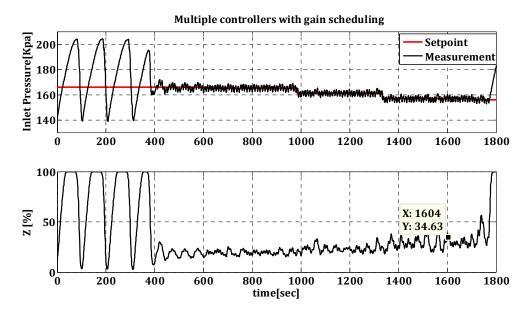
Figure 5.14: Results of gain scheduling using four PI controllers. When the system was switched into the fifth controller the instability was appeared; meaning that the maximum level of stability was reached with four controllers tuned by simple online tuning rules. The controllers have been able to move the bifurcation point from Z=16% up to Z=35%.
