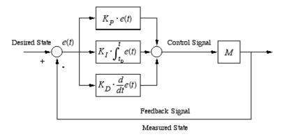
Figure 2.9: A typical PID control structure
