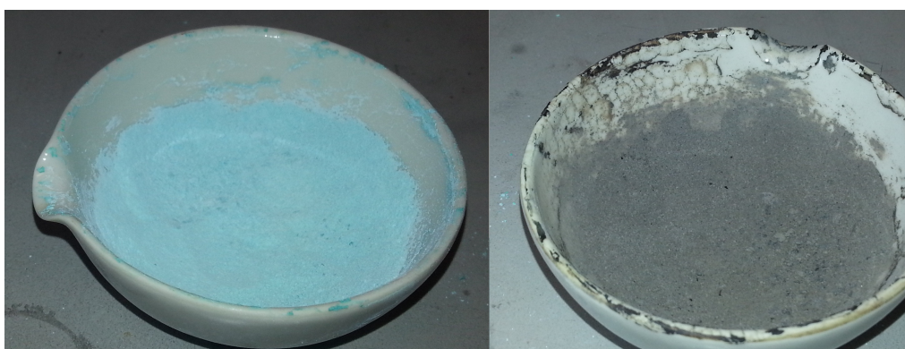
Figure 19: The picture shows how the dried catalyst looked before (left) and after (right) the calcination process.
