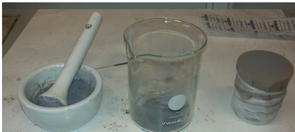
Figure 20: This is the equipment used for crushing and sieving.
