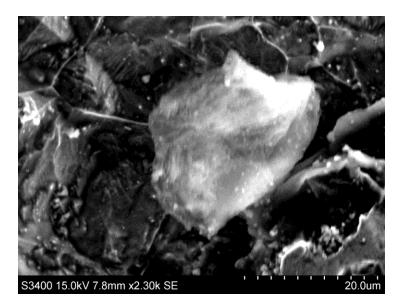
Figure 8-26. SEM showing typical geothite phase of corrosion product
