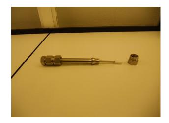
Figure 6-1. Picture of sample in the cylinder, showing also the Teflon cover at the tip of the metal specimen
