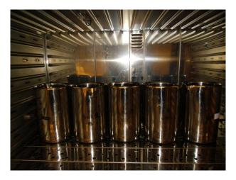
**Figure 7-5.** The inside of the Memmert ®600 thermostat chamber at 135°C with the containers for the 5 different weeks of exposure shown.
