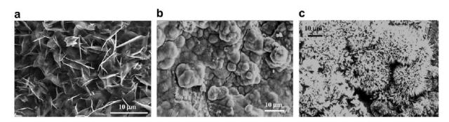
**Figure 6-5.** SEM images showing different phases and forms of corrosion products (S.W. Dean, D. Knotkova et al. 2010; de la Fuente, Díaz et al. 2011)
