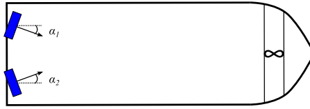
Figure 7.4: Biasing of main thrusters placed at the stern
