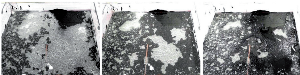
Fig. 3. The air gaps, the white spots in the photo, which became visible during the end of the melting process of compressed snow. The figure shows the appearance of the air gaps after around 2 h and the change of the surface area of the air gaps within a time frame of 10 min.
