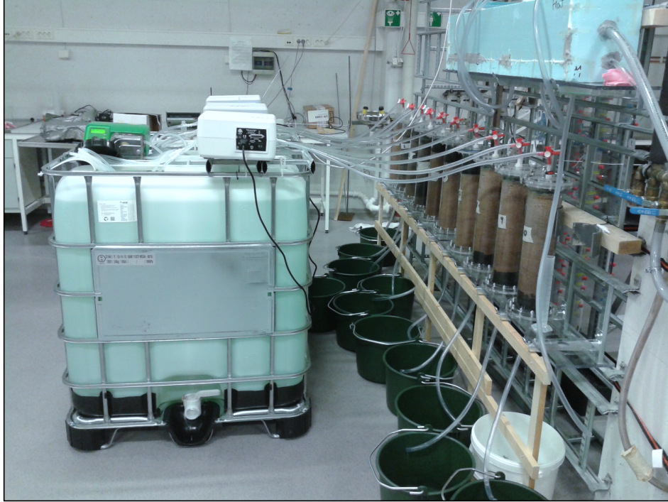
Figure 4. Column setup during the toxic metal pump into the adsorbent amended filters.
