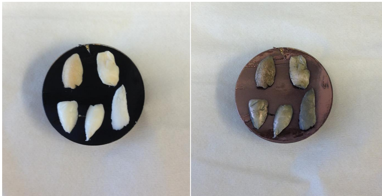
Figure 2.14.1: Pieces from the edges of the freeze-dried gels, mounted with carbon tape on SEM sample holder, pre- (left frame) and post-coating (right frame) with gold for 45 s.
