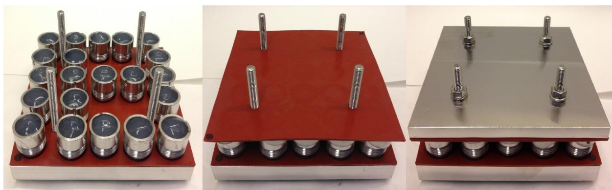
Figure 2.7.1: The setup with the casting molds of stainless steel used in this project for preparing cylindrical gels of crosslinked MFC. The molds were filled with positive/convex menisci to obtain gels with equal volume, as the surplus of sample was pressed out of the molds when the silicone seals were tightened.
