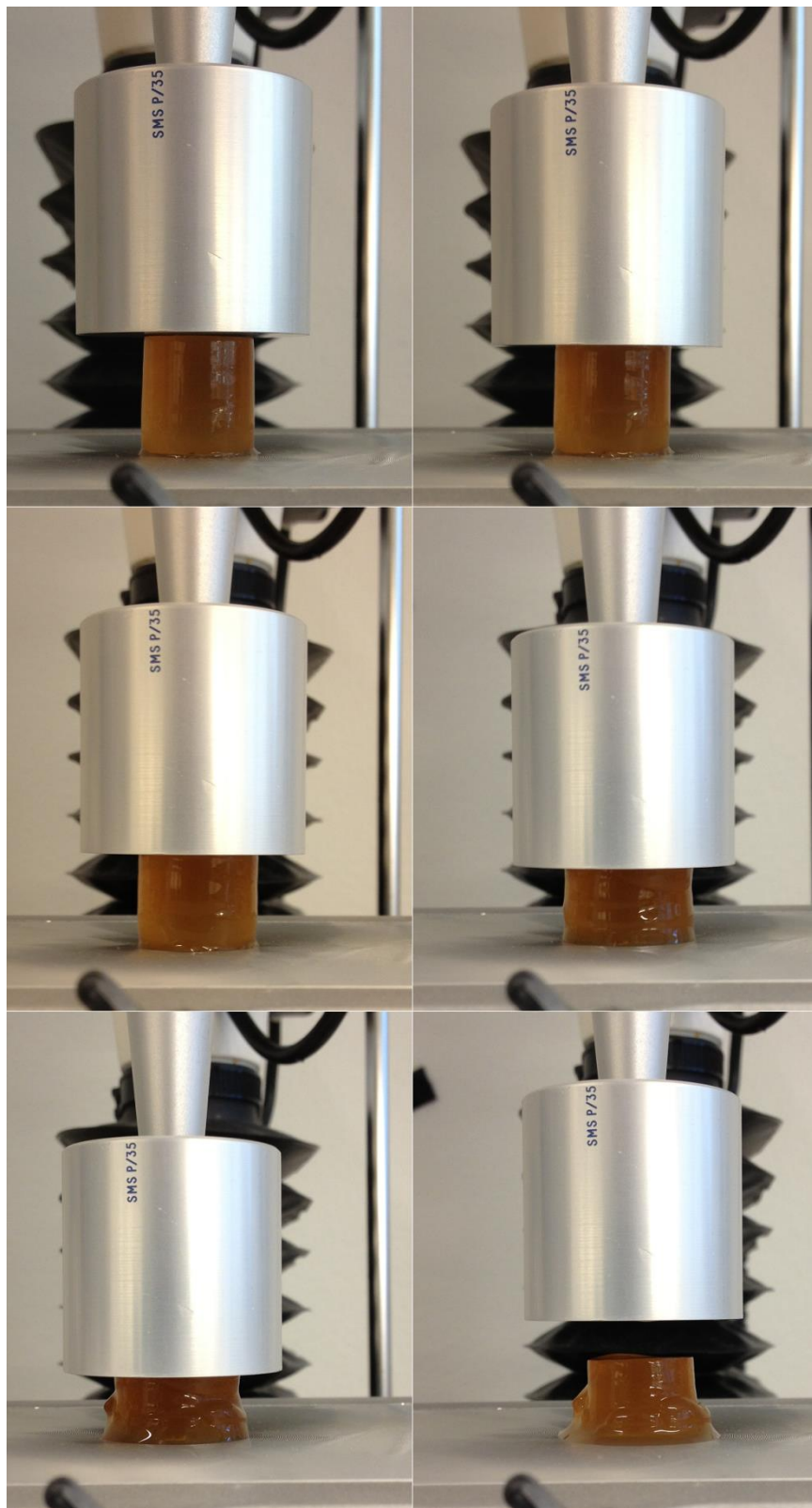
Figure C.2: Longitudinal compression (8 mm compression after a trigger force of 1 g was reached) of one gel with HMDA (3.05 mmol/g MFC). The compression is recorded in one of the curves in Figure C.4.
