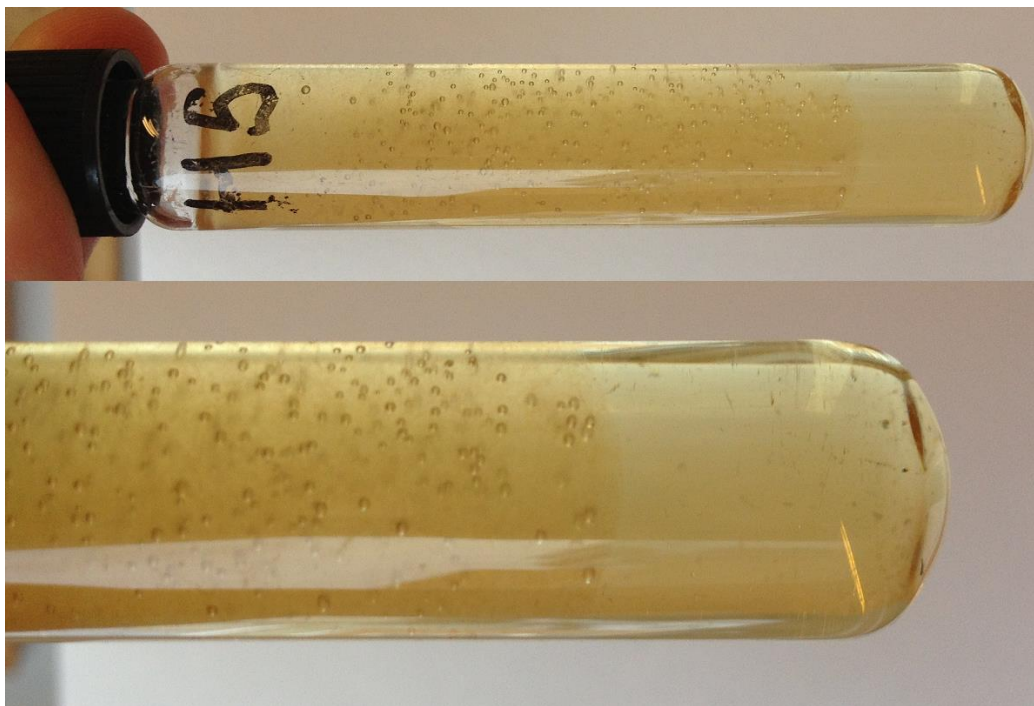
Figure 3.2.1: Test tube containing 0.25% MFC and 3.05 mmol HMDA/g MFC (H50) after approximately 20 hours in a water bath at 80° C. Even containing >99.5% water, the test tube could be turned sideways and upside down without observable viscous behavior in the gel. Notice the phase separation where water has been excreted in the bottom of the test tube. Also notice the air bubbles captured in the gel matrix. These were probably introduced during the mixing of the crosslinker solution into the MFC suspension. The color change from the original slightly bluish grey to a brownish yellow seemed to correlate with the amount of HMDA.
