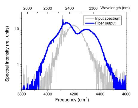
Figure 3.Spectra (log scale) of femtosecond pulses after propagation in 1.5 m highly Ge-doped fiber.
