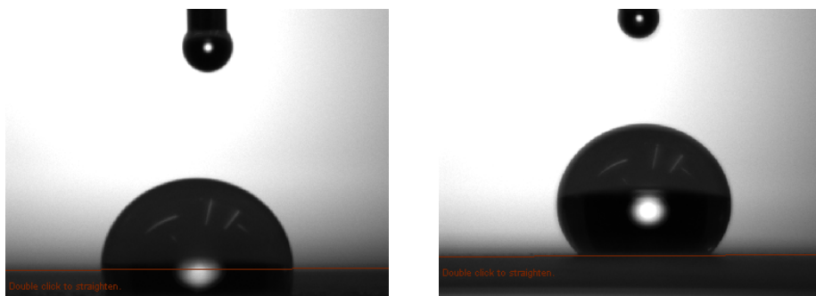
Figure 5.37: Droplets on coatings without graphite/CB. The left image is without Zonyl content, and the right image is with 8.3 vol% Zonyl.
