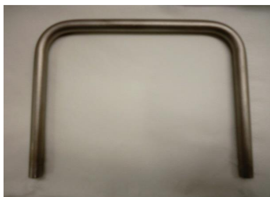
Figure E.1: Sandblasted stainless steel tube used in experiments.
