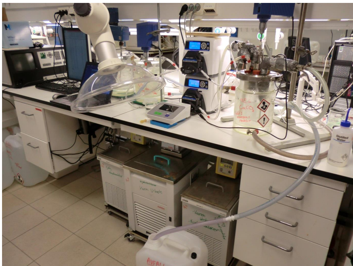
Figure E.3: Experimental setup with pre-coolers, logging, pump, reactor and thermostatic units.
