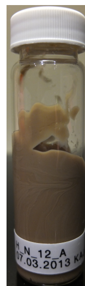
Figure 13 – Very strong emulsions were formed when mixing the crude oils with NaCl brine of pH 12. This is an sample made from crude oil H.
