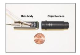
Figure 2.1.4 $^6$  – the size of the device in relation to US 1-cent coin
