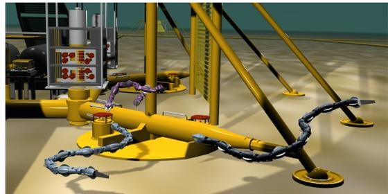
Fig. 1: Underwater snake robots capable of both inspection and light intervention tasks.
