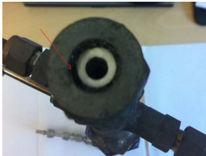
Figure 4.2.3 Picture of connection quencher to ceramic tube after use. Red arrow points to a cavity/hole in grafoil sealing.
