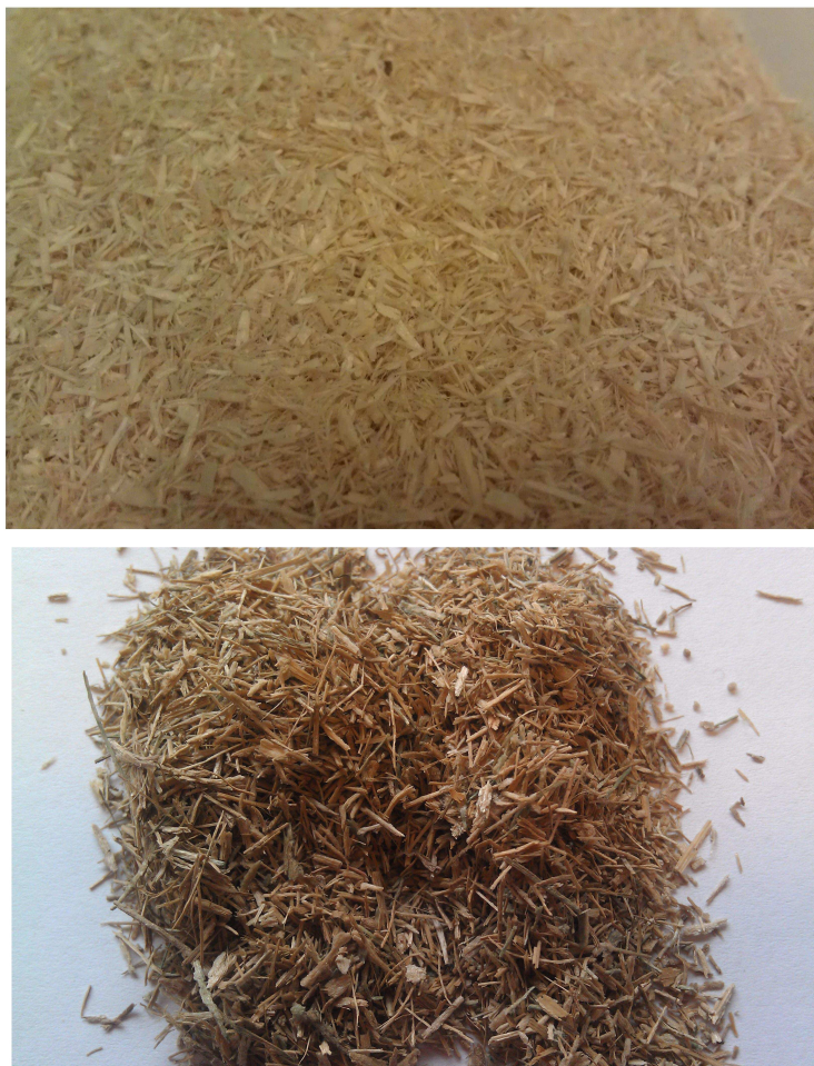
Figure 13: The raw materials used in this work, spruce (above) and bagasse (below).
