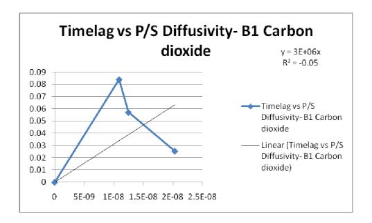
**Figure 6.3.13:** Comparison of the two diffusivities from time lag method and P/S (B1-CO<sub>2</sub>)
