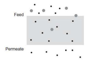
Figure 4.1.1: Solution diffusion transport mechanism [4]
