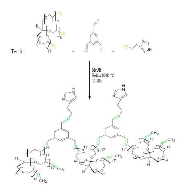
Figure 6.2.4: T3 polymer synthesis reaction [16].
