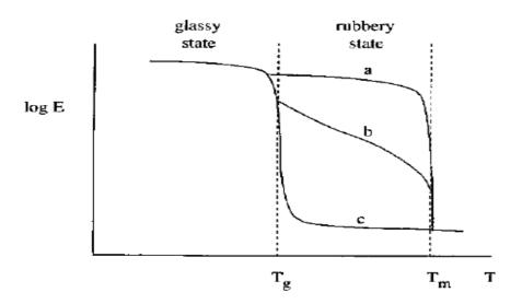
**Figure 3.3.3:** Tensile modulus of i) crystalline ii) semi crystalline iii) amorphous polymer as a function of the temperature [12].
