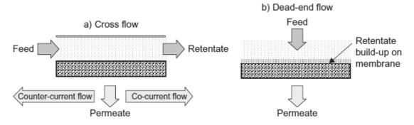
Figure 3.1.1: Cross flow (a) and dead flow (b) membrane configurations [4]
