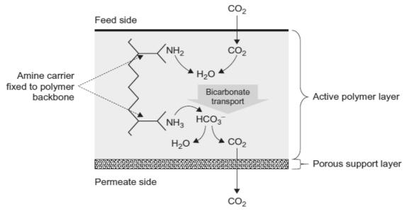
**Figure 4.4.2:** Facilitated transport of CO<sub>2</sub> through membrane (fixed carrier – amine groups) [19]
