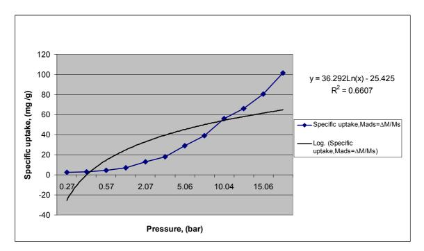
**Figure 6.3.9:** Specific uptake of  $CO_2$  as a function of pressure at  $25^{\circ}C$  in PDMS
