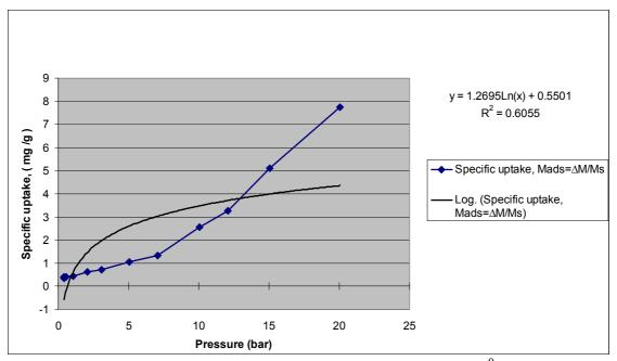
**Figure 6.3.2:** Specific uptake of  $N_2$  as a function of pressure at 25<sup>o</sup>C in B0-PDMS (50-50 %).
