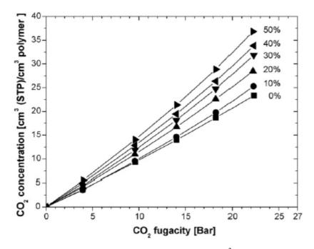
**Figure 2.3.3:** CO2 concentration (cm3 (STP)/cm<sup>3</sup> polymer) as a function of CO2 fugacity at  $35^{\circ}$ C for PABX<sup>®</sup> 1657/PDMS-PEG blend membranes with different PDMS-PEG additive blend ratio [7].
