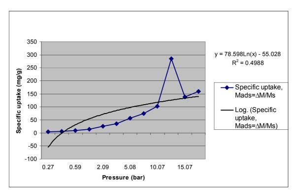
**Figure 6.3.11:** Specific uptake of  $CO_2$  as a function of pressure at 25<sup>o</sup>C in T3
