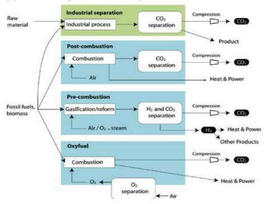
**Figure 1.1.2:** Schematic representation of capture systems. Fuels and products are indicated for oxyfuel combustion, pre-combustion (including hydrogen and fertilizer production), post-combustion and industrial sources of CO2 (including natural gas processing facilities and steel and cement production) (from CO2CRC) [3].
