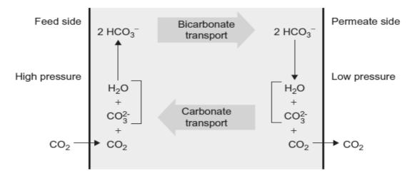
**Figure 4.4.1:** Facilitated transport of CO<sub>2</sub> in supported liquid membrane (mobile carrier-carbonate) [4]
