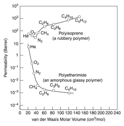
**Figure 3.4.1:** Permeability of a rubbery and a glassy polymer as a function of molar volume [13].
