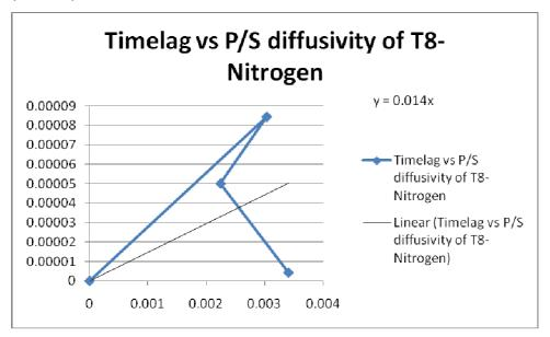
**Figure 6.3.16:** Comparison of the two diffusivities from time lag method and P/S (T8-N<sub>2</sub>)
