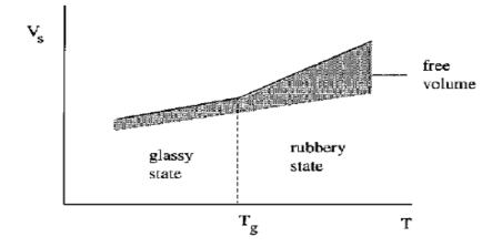
Figure 3.3.2: specific volume and free volume as a function of temperature [12]
