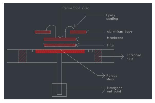
Figure 5.4.2: Cross section of the membrane module (lower flange).
