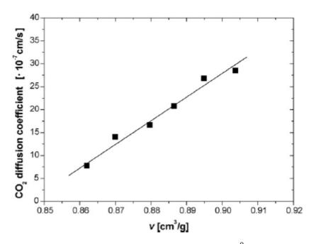
**Figure 2.3.4:** Diffusion coefficient of  $CO_2$  at  $35^0C$  as a function of the polymer specific volume for PABX<sup>®</sup> 1657/PDMS-PEG blend membranes [7].
