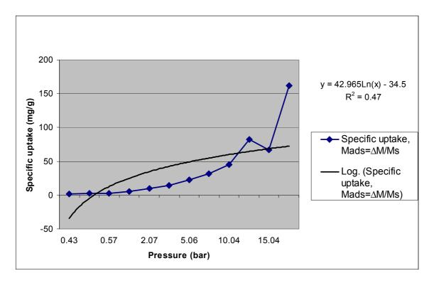
**Figure 6.3.8:** Specific uptake of  $CO_2$  as a function of pressure at  $25^{\circ}C$  in B0-PDMS
