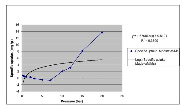
Figure 6.3.5: Specific uptake of  $N_2$  as a function of pressure at  $25^{0}$ C in T3
