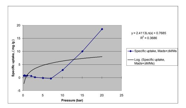
Figure 6.3.6: Specific uptake of  $N_2$  as a function of pressure at  $25^{0}$ C in T8
