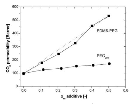
**Figure 2.3.1:** Pure gas  $CO_2$  permeability at  $35^0C$  and 4 bar as a function of additive mass fraction of blend membranes with (i) PDMS-PEG (ii) PEG<sub>200</sub> [7].
