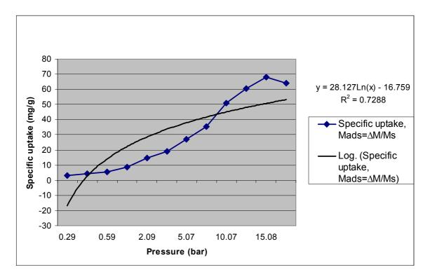
**Figure 6.3.10:** Specific uptake of  $CO_2$  as a function of pressure at  $25^{\circ}C$  in B1
