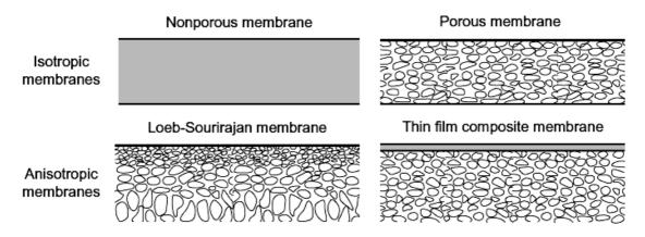
Figure 3.2.1: Different types of membranes on the basis of their physical structure [4].
