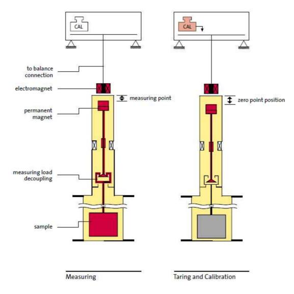
Figure 5.3.2: Automatic calibration and tarring of magnetic suspension balance (MSB) [15]
