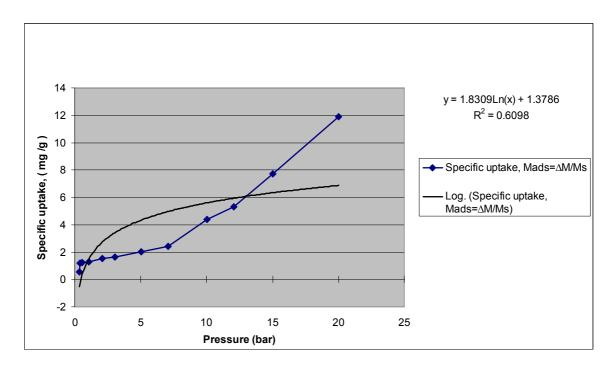
Figure 6.3.3: Specific uptake of  $N_2$  as a function of pressure at 25<sup>o</sup>C in PDMS
