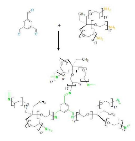
Figure 6.2.3: B1 polymer synthesis reaction [16]
