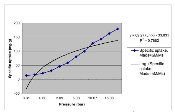
**Figure 6.3.12:** Specific uptake of  $CO_2$  as a function of pressure at 25<sup>o</sup>C in T8
