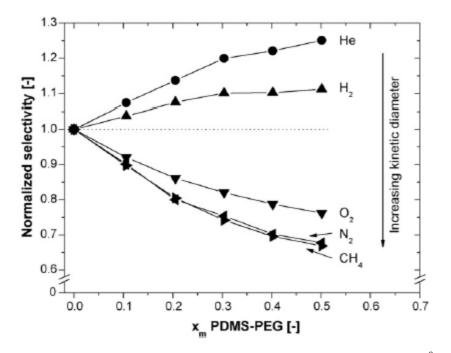
**Figure 2.3.2:** Normalized pure  $CO_2$ /light gas selectivities at  $35^0$  C and 4 bar as a function of additive mass fraction of blend membranes with PDMS-PEG [7].
