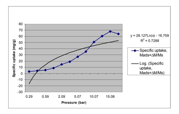
Figure 6.3.4: Specific uptake of  $N_2$  as a function of pressure at  $25^{\circ}$ C in B1
