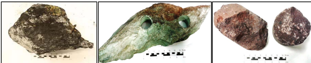
Figure 6: Photo of the three rock type, from left to right; alum shale, greenschist and tuff.
