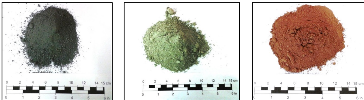
Figure 7: Photos of prepared dust powder for free swelling, swelling pressure and XRD analysis, from left to right; alum shale, greenschist and tuff.
