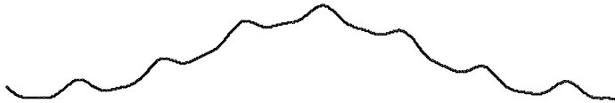
Figure 5.3 Eulerian spatial snapshot of the surface \eta(x) in two-component waves according to Eq. (4.39), with the same component parameters as in Figure 5.1 and Figure 5.2.
