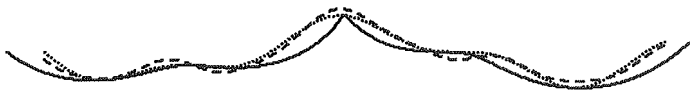
Figure 5.4 Eulerian spatial snapshot of the surface \eta(x) in two-component waves. \lambda_{\text{long}}/\lambda_{\text{short}} \approx 3 , ka_{\text{long}} = ka_{\text{short}} \approx 0.4 . The solid line represents the parametric form equivalent to the case in Figure 5.1, the dotted line is equivalent to the case in Figure 5.2, and the dashed line is equivalent to the case in Figure 5.3.
