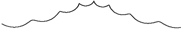
Figure 5.1 Eulerian spatial snapshot of the surface \eta(x) in two-component waves according to Eq. (5.1). \lambda_{\text{long}}/\lambda_{\text{short}} \approx 8 , ka_{\text{long}} \approx 0.2 , ka_{\text{short}} \approx 0.4 .
