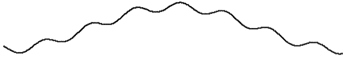
Figure 5.2 Eulerian spatial snapshot of the surface \eta(x) in two-component waves according to Eq. (5.4), with the same component parameters as in Figure 5.1.
