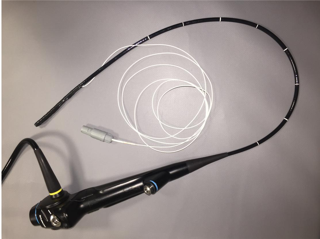
Figure 4: The bronchoscope with a position tracking sensor mounted close to the tip.
