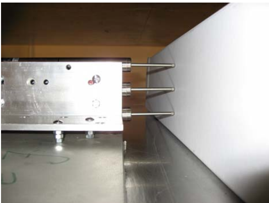
Figure 3. Three displacement transducers measuring the outward buckling of the long wall before the start of a BCT test.
