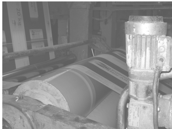
Figure 3.1: Glue applicator roll.
