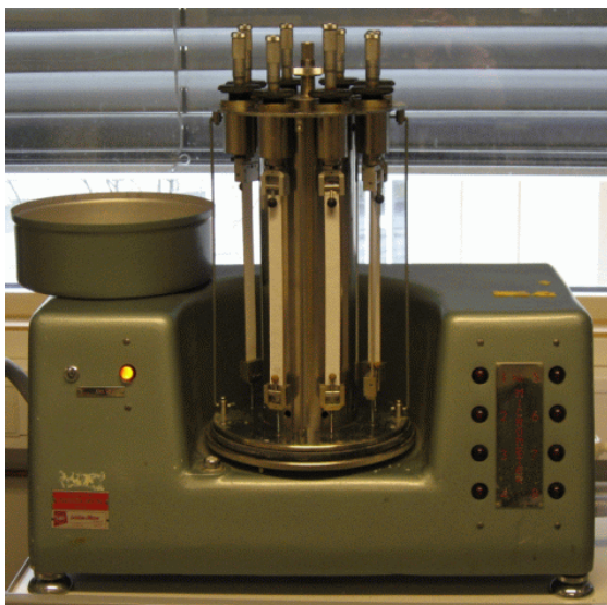
Figure 2. The micrometer tester used in hygroexpansion tests without the climate preserving cylinder around the clamps.
