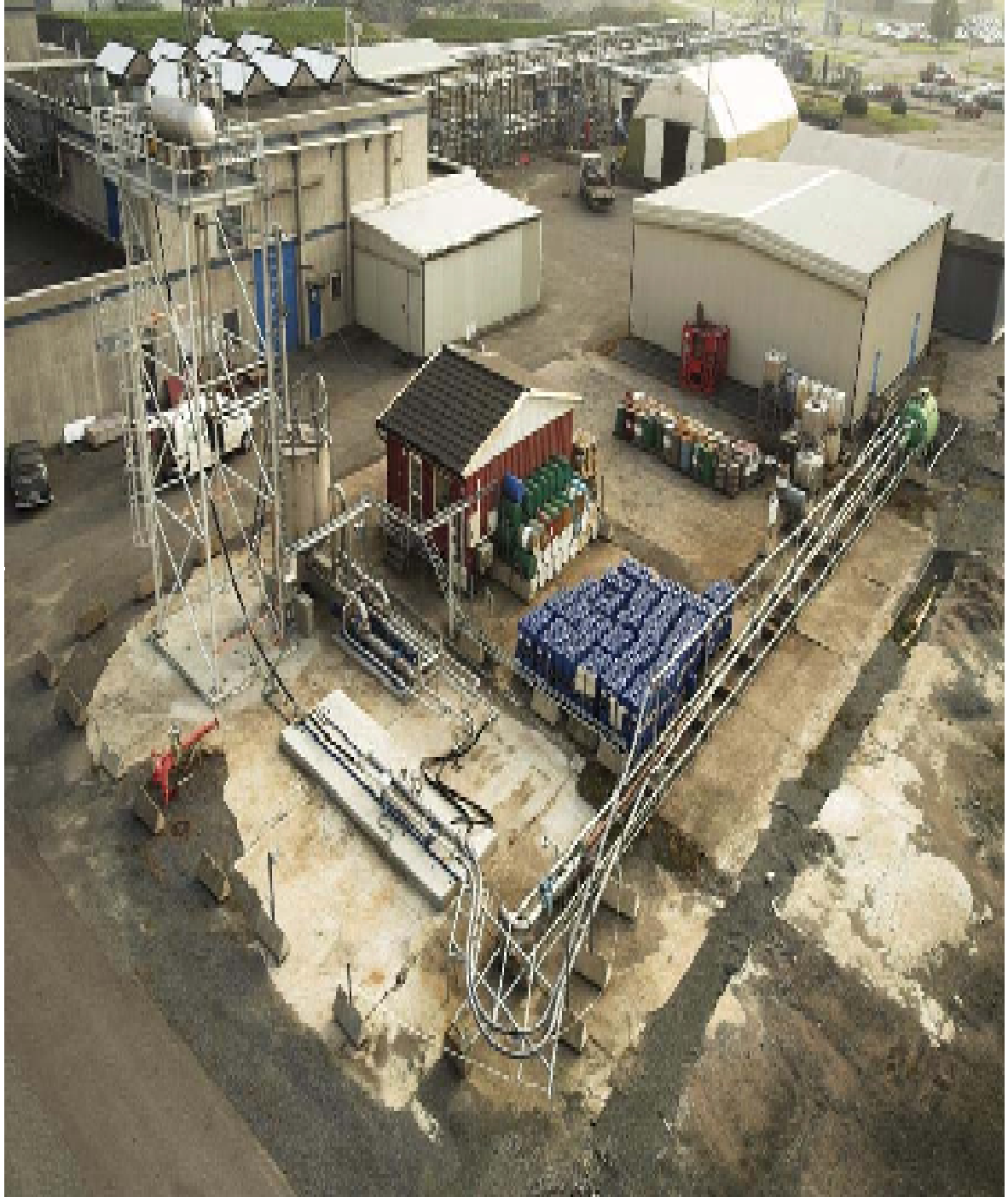
Figure 1.4: A birds-view perspective of the medium-scale riser rig at StatoilHydro Research Center in Porsgrunn
