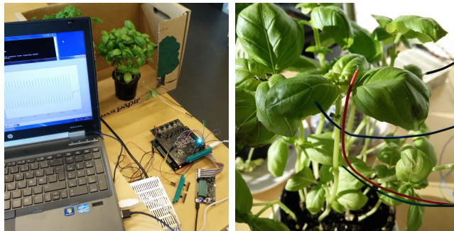
(a) Mecobo board connected to Basil plant setup. (b) Basil and needle electrodes setup.
