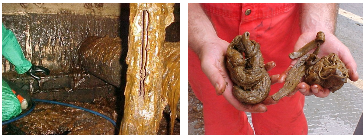
Figure 3.1: Naphthenate deposits in a separator vessel during clean out (left picture). Naphthenate collected from the separator (right picture). Reproduced with permission from OilPlus, UK.
