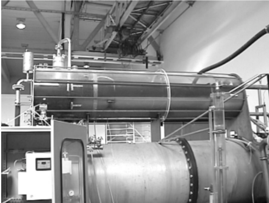
Figure 2.5: Picture of the pilot separator during an oil continuous run with fluid system 3. The dispersion band is clearly distinguishable as a gray layer between the transparent bulk liquid layers. Below the pilot model, the feed tank can be seen as well as the oil-in-water monitor. Flow direction is from right to left.
