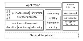
Figure 4: Building blocks of an MSN architecture.
