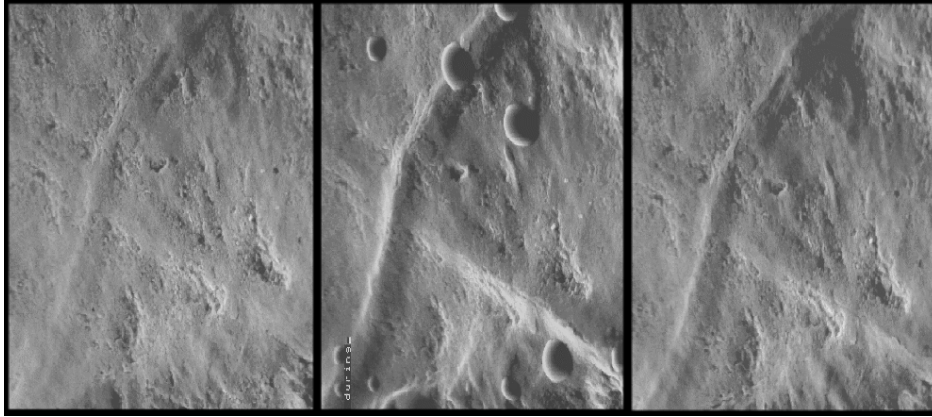
Figure 2.5 ESEM images of a coated supercalendered paper before (left), during (middle) and after (right) moistening [134].
