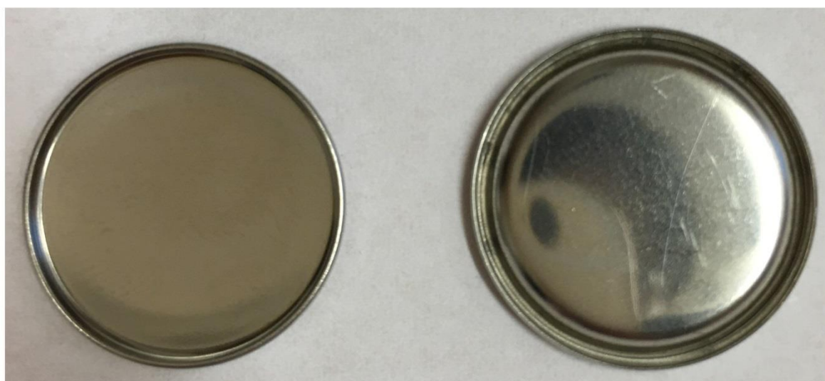
Figure S2. The photographs of a dissembled coin cell after 1000 cycles charge/discharge. The cell was washed by THF in order to clean the residual electrolyte and dried 2 hours at room temperature under vacuum.
