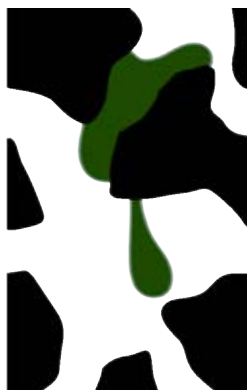
Figure 4: 3-6 mm droplets flowing along coke particles
