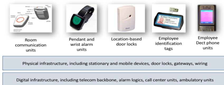
**Figure 1. The digital and physical infrastructure of the surveillance system.**
