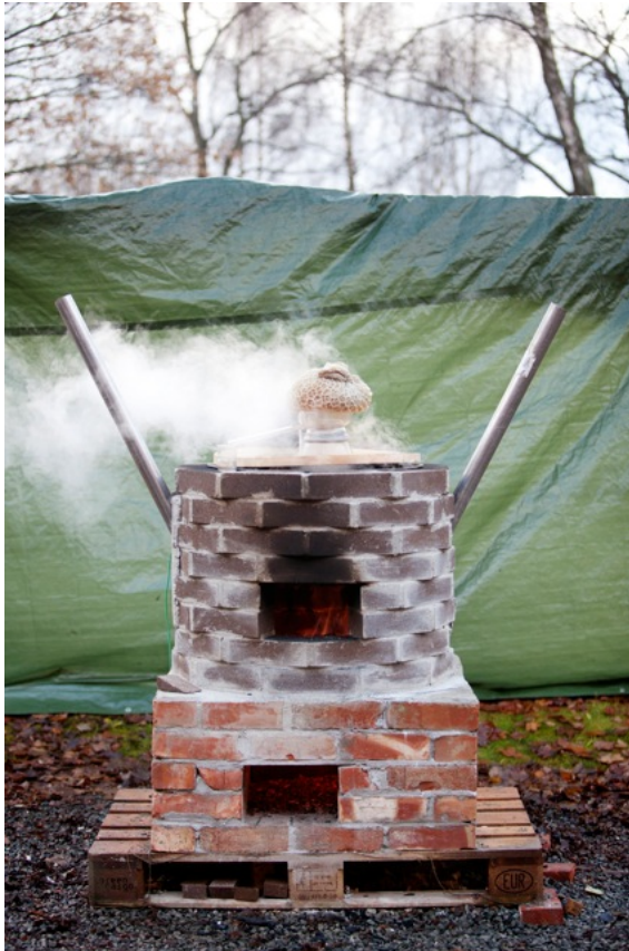
Figure 7.2: The completed furnace with a cow's reticulum as an improvised moor's head
