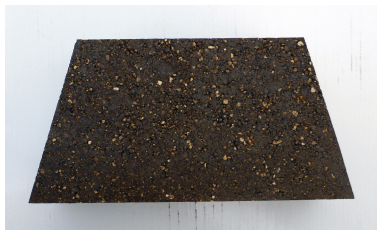
Figure 7.6: Trapeze shaped bricks were made by cutting standard bricks to shape
