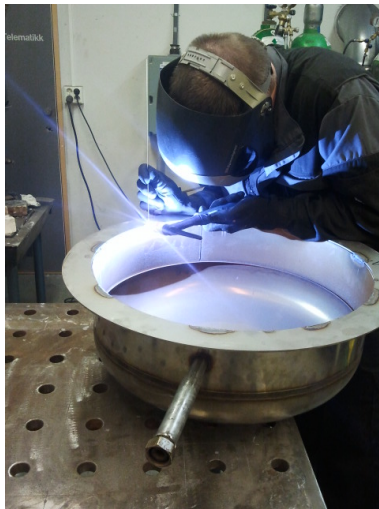
Figure 7.8: The rim for the kettle is welded on by Robert Karlsen at the University workshop
