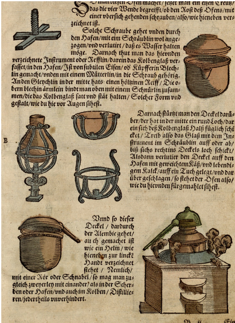
Figure 7.20: A devise for mounting a cucurbit in a waterbath
