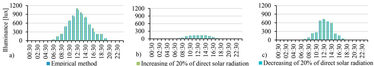
Fig. 3. Comparison between the illuminance values carried out from the analysis of daylight autonomy conducted in *DIVA-for-Rhino* for (a) 17<sup>th</sup> of April, (b) 13<sup>th</sup> and (c) 18<sup>th</sup> of March and for the three methods: empirical, increasing and decreasing of 20% of the direct solar radiation.
