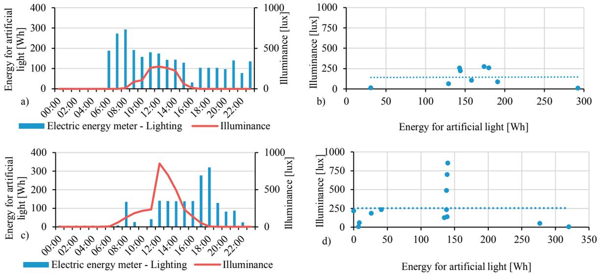
Fig. 4. The hourly illuminance values and energy for artificial light (a) and the correlation between illuminance level and energy for artificial light on the 11<sup>th</sup> of February (b) and for the 15<sup>th</sup> of March (c) and (d). The dotted line indicates the period considered for the correlation.
