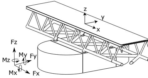
Figure 6: Sketch of the modelling of the wave forces on the pontoons.
