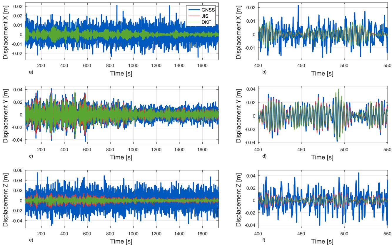
Figure 18: Estimated displacement history in recording 1 compared to GNSS measurements.
